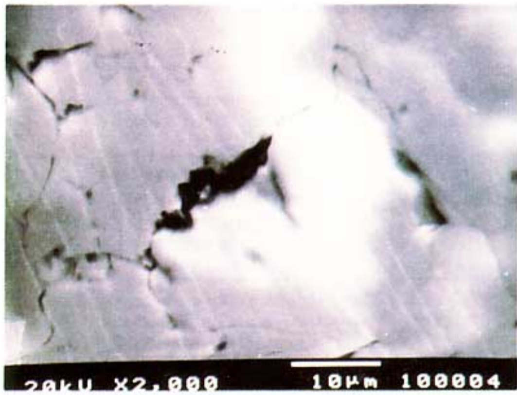
Fig.3. Compact interlocking grain boundaries of natural jadeite. (x2,000)
