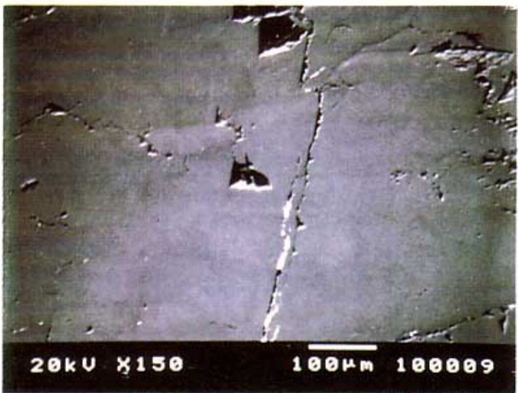
Fig.4. Electrical charging (bright white line) of polymer infilled grain boundaries and defects on the surface of a bleached polymer-impregnated jadeite. (x150)
