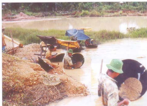
Fig. 3. Washing the sandy gem diamond gravels using a pan made of black iron wood called dulang .
